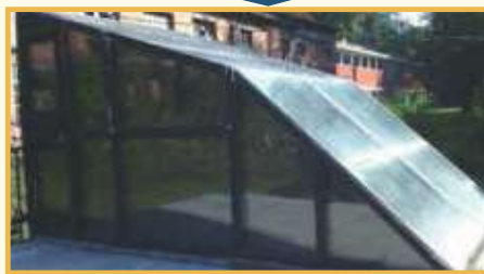
Head based storage Solar Kiln
