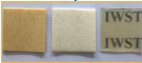
Natural wood (Left most), Lignin modified wood (middle) and Transparent wood (right most) placed on a paper with letters "IWST"
